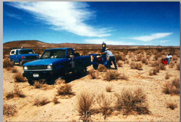
Seismic refraction survey using a 24-channel Geometrics seismograph and Dynasource vacuum-accelerated weight drop as the energy source
