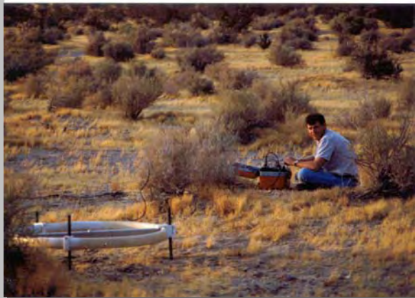
Time-domain electromagnetic survey using a Geonics EM47 ProTEM system
