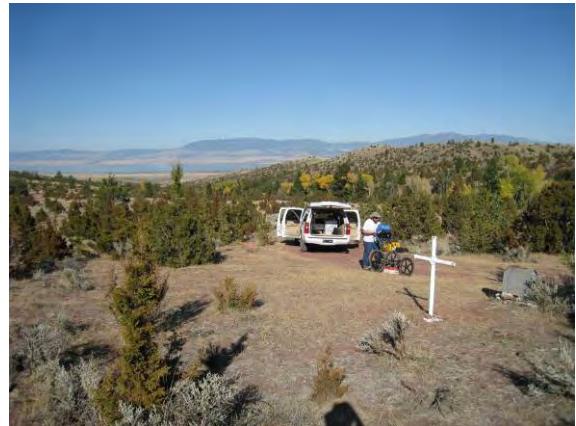
GSSI SIR-3000 GPR survey at Burial 1
