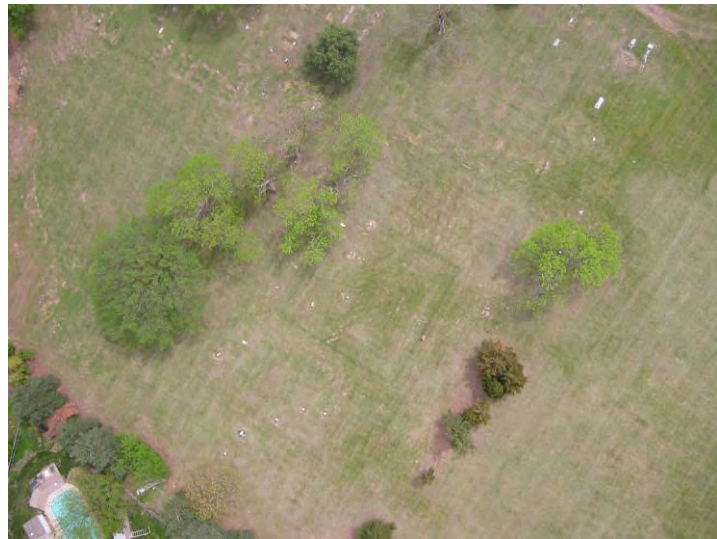
Kite Aerial Photography over project site. Aerial photography reveals vegetative tonal difference synonymous with grave patterns and orientations.
